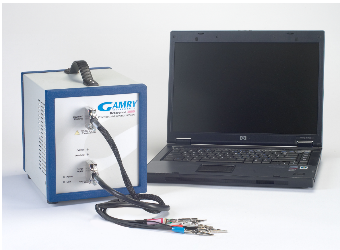
Installed Potentiostat with Cell Cable Attached
